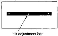
6. Press or boto adjust the picture tilt until left and right side of tilt adjustment bar is parallel to the bottom of picture frame (if necessary).
